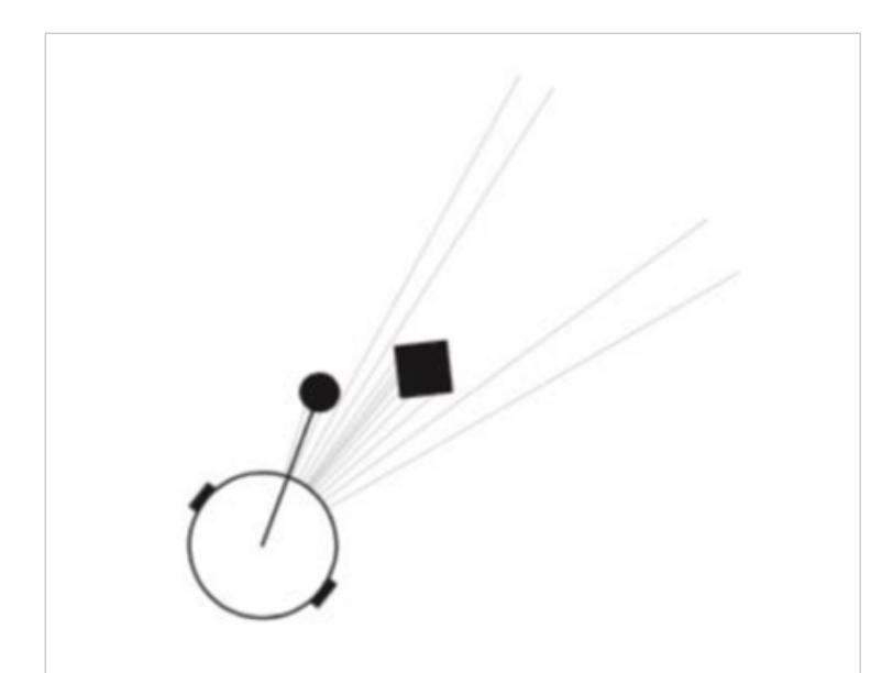
Figure 1: Basic design of a visually-guided agent. The agent (large circle) has an eye (gray lines), two motors (filled rectangles) and a transparent arm (solid line) with an opaque hand (filled circle). The arm can rotate about the center of the agent and extend or retract along its length. The hand can rotate about its point of attachment with the arm.
